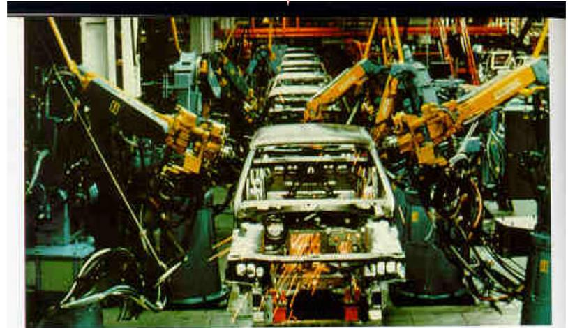
Industrial robots spot weld automobile bodies on an assembly line.
