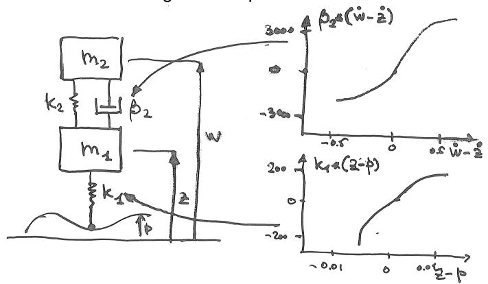
$m_2$  : overall mass of the body of car with passengers, engine, etc.
