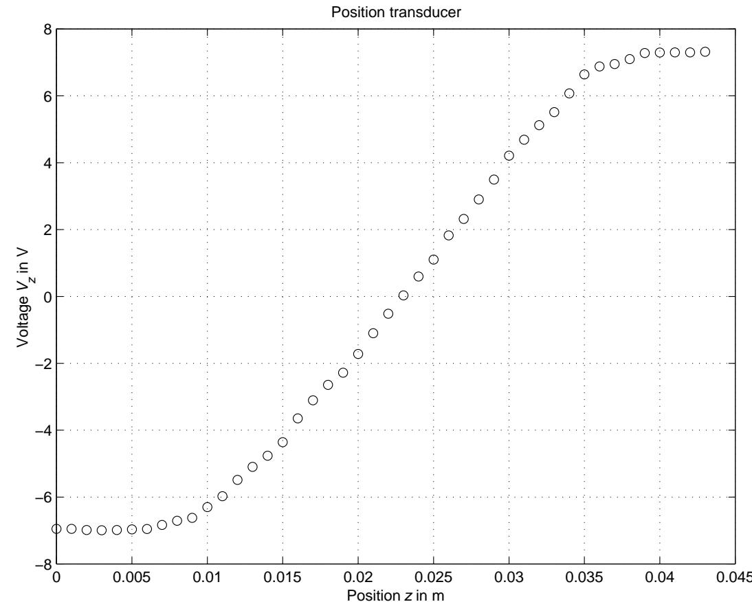
The static characteristic of the position-voltage transducer is nearly linear in the range between 1.3 e 3.5 cm  $\Rightarrow$  the characteristic can be linearly approximated by:
