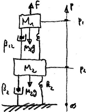
$$\begin{aligned} M_1 &= 2 \text{ kg}, \quad M_2 = 5 \text{ kg}, \\ k_{12} &= 30 \text{ N/m}, \quad k_{12} = 10 \text{ N/m}, \\ \beta_{12} &= 20 \text{ Ns/m}, \quad \beta_{12} = 10 \text{ Ns/m}, \\ g &= 9.81 \text{ m/s}^2 \end{aligned}$$
