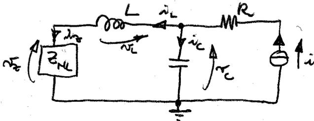
$$\begin{aligned} v_2(t) &= \alpha i_2(t) + \beta i_2^3(t) \quad (5) \checkmark \\ x(t) &= \begin{bmatrix} i_L(t) \\ v_C(t) \end{bmatrix} = \begin{bmatrix} x_1(t) \\ x_2(t) \end{bmatrix} \\ u(t) &= [i(t)] \end{aligned}$$
