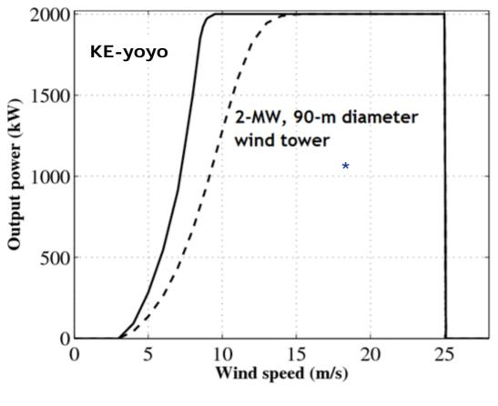
Due to wind variability, a wind generator is able to produce in average only a fraction of its rated power, called "Capacity Factor":
