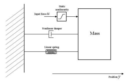
Figure 1: Nonlinear mass-spring-damper system.
